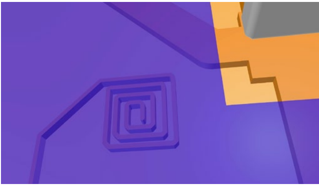
Figure 4: Zooming past the transition between land and trace we see a small UHDI trace emerge. What it will be used for (application and cost) is yet to be determined, but it is good to know that the manufacturing capability is there to support the requirement when an application arises.
